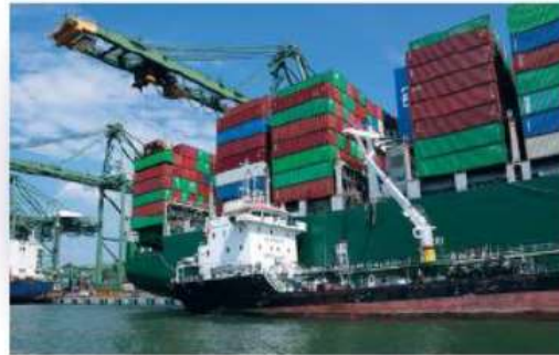
Ship-to-ship bunkering with cargo handling (SIMOPS)
