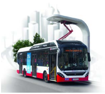
eBus charging systems
