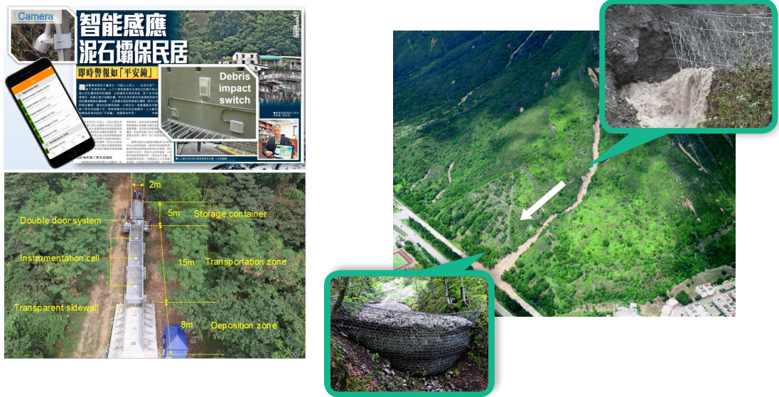
FIGURE 3-3 NEW LANDSLIDE BARRIER SYSTEM BY GEO/CEDD-HKUST
