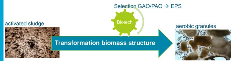
Operation of Nereda results in stable granulation thanks to
